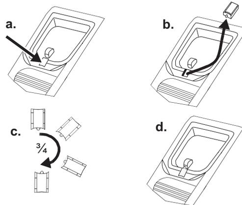
**FIGURE 7 Removing, Rotating, and Replacing the Handset Retainer**
