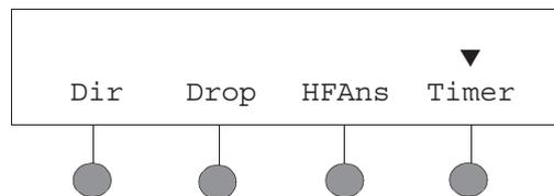
The **top line** of each softkey feature menu screen shows you the status of each of the four features. An arrow appears above the feature name or abbreviation if that feature is active. In the above example, the arrow above the Timer feature indicates that feature is active.
