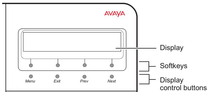
**FIGURE 4** The Display, Softkeys, and Display Control Buttons
